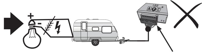
**Kurzschluss/Short circuit fault on PIN 7, 8 oder/or 10**
